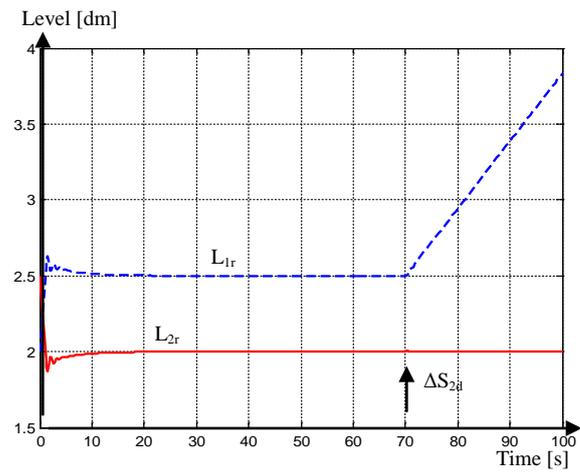
Fig. 11 The level  $L_{1r}$  and  $L_{2r}$  for  $\Delta S_{2d}=0.1$
