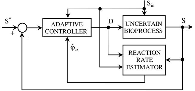
Fig. 1. Scheme of the adaptive closed-loop controlled system
