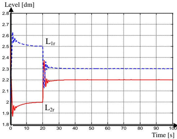
Fig. 3 The level  $L_{1r}$  and  $L_{2r}$  in normal condition to the change of the prescribed size
