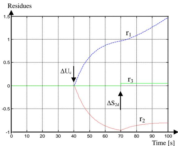
Fig. 14 The residues  $r_1$ ,  $r_2$  and  $r_3$  for  $\Delta U_d=0.1$  and  $\Delta S_{2d}=0.05$
