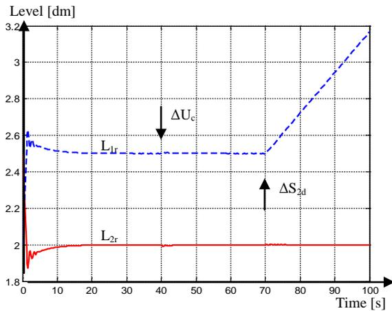
Fig. 13 The level  $L_{1r}$  and  $L_{2r}$  for  $\Delta U_d=0.1$  and  $\Delta S_{2d}=0.05$
