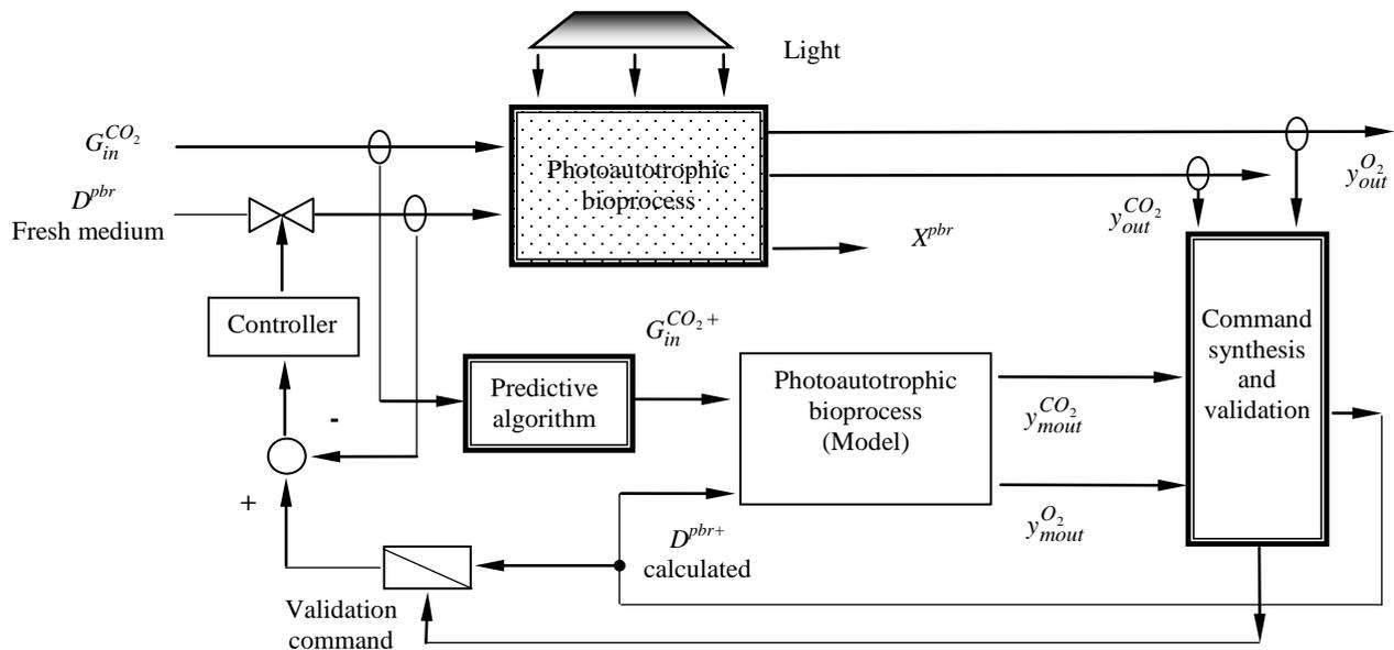
Fig. 3. The structure for control system with predictive algorithm.
