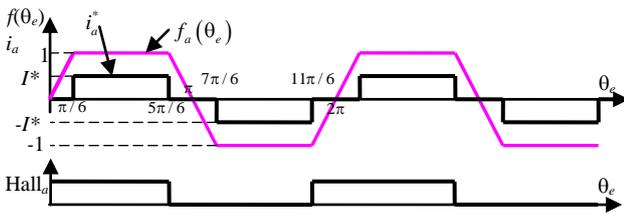
Fig. 1. The waveforms for the phase a.
