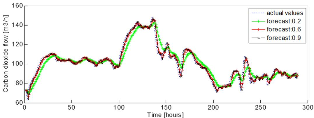
Fig. 4. The values of  $CO_2$  flow with predictive algorithm (simulation).
