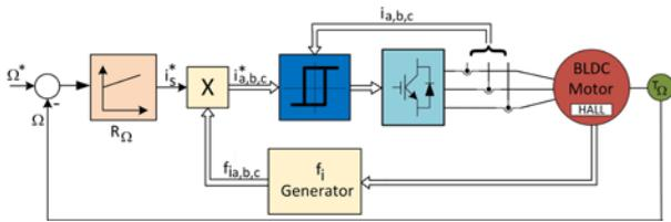
Fig. 6: Principle diagram for the preset currents command
