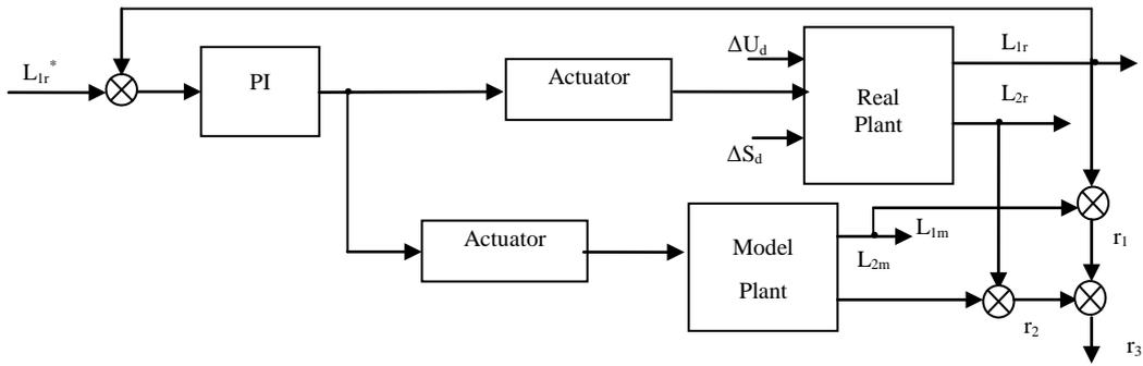
Fig. 2 The fault detection structure
