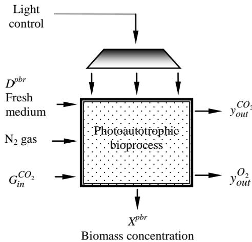
Fig. 2. The structure for the photoautotrophic bioprocess.
