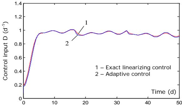
Fig. 6. Profile of control input  $D$  – case 1
