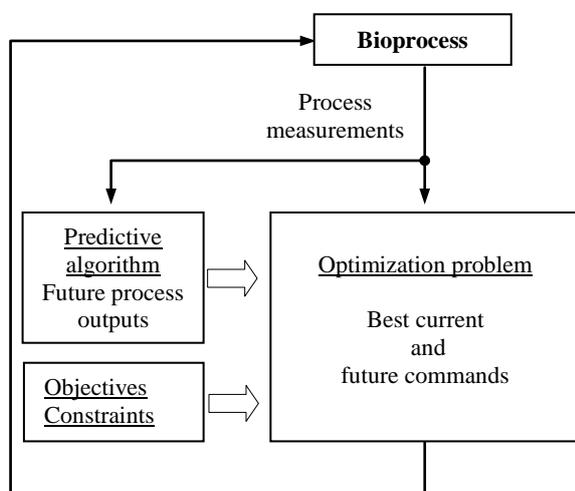
Fig. 1. The structure of the predictive control system.
