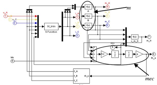
Fig. 2: The Simulink model of the BLDC with S-function.
