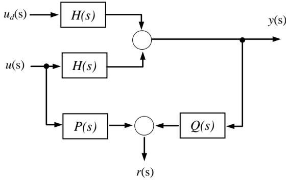
Fig. 4. The generation of the residue.
