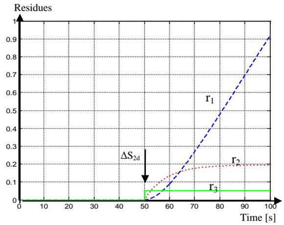
Fig. 10 The residues  $r_1$ ,  $r_2$  and  $r_3$  for  $\Delta S_{2d}=0.05$
