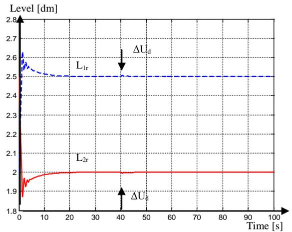
Fig. 5 The level  $L_{1r}$  and  $L_{2r}$  for  $\Delta U_d=0.1$
