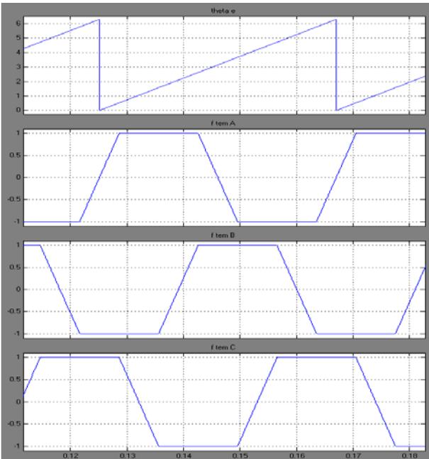
Fig. 4: The reference back emf functions  $f_a, f_b, f_c$ .
