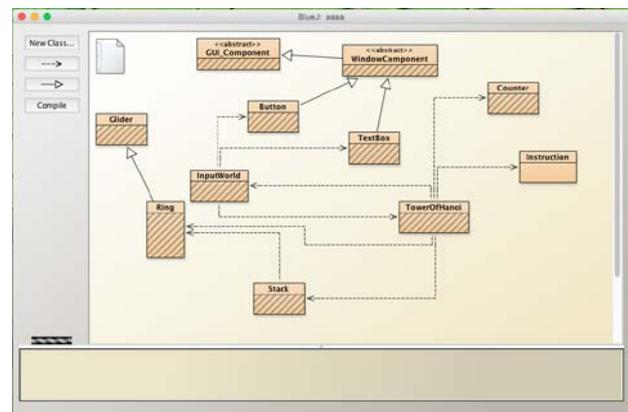
Fig. 4. UML diagram of our project in BlueJ.
