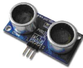
Fig. 2 – The distance sensor HC-SR04
