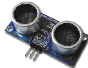
Fig. 2 – The distance sensor HC-SR04
