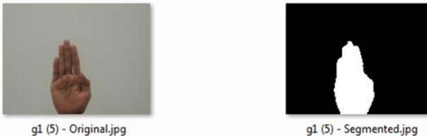
Figure 7 Otsu's Binarization Results
