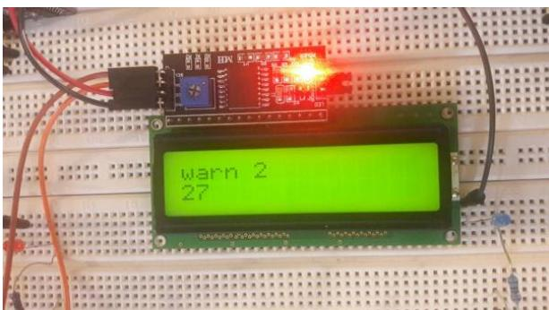
Fig.4 The message displayed on a possible Level 2 collision
